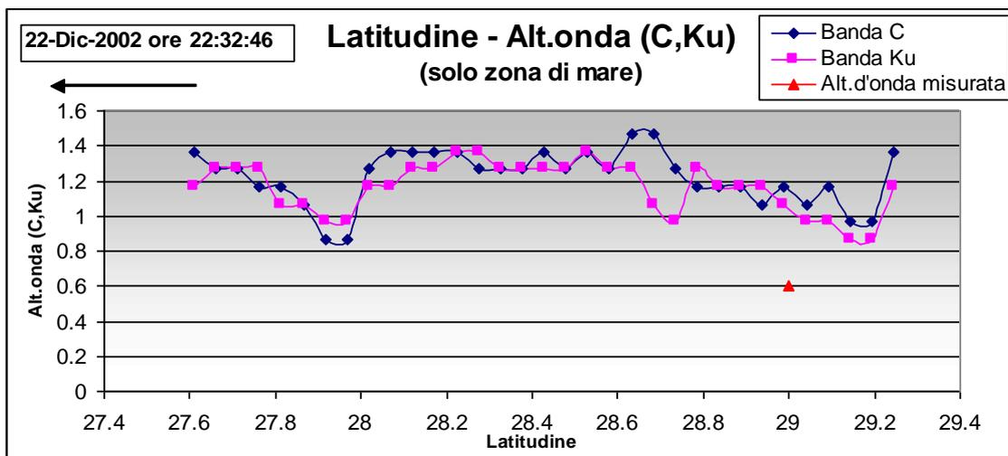
**Figure 2: December 2002 Significant wave height form Topex altimeter-**
