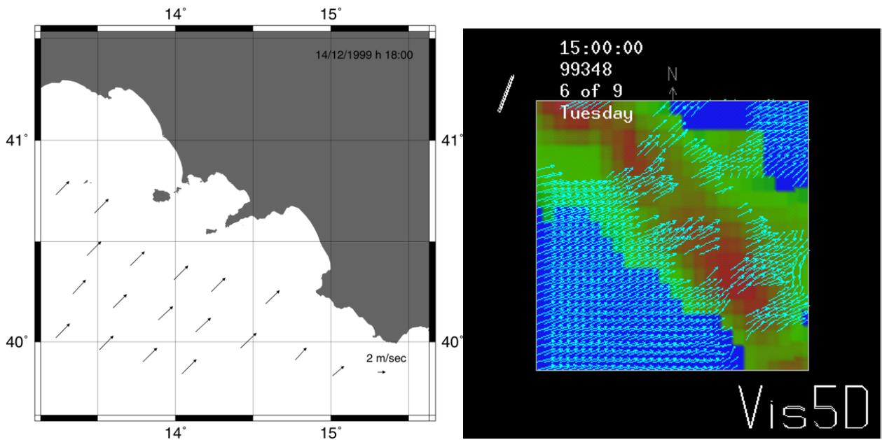
Figure X: Wind velocity vectors as computed with a Local Area Model and measured by satellite scatterometer
