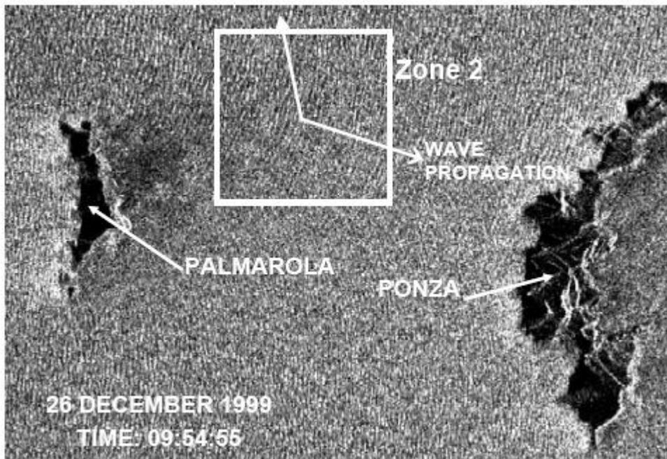
The image texture is clear enough to detect the wave fronts, and to evaluate the wave direction, both for location 1 and 2. Power spectra of the pixel intensity values were also calculated (figures 3a and 4a).
