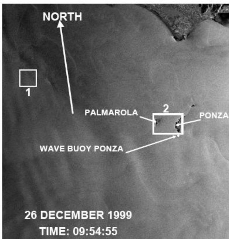
Wave parameters measured at 09:00 the Ponza buoy (about 1 km south of the islands) are:  $H_s = 1.70$  m,  $T_m = 5.3$  s,  $T_p = 6.7$  s, propagation direction =  $66^\circ$ . Wind direction, as measured from the local anemometer in the Ponza island itself is  $250^\circ$  and its 10 meter velocity  $V_{10}$  is  $6.5 \text{ ms}^{-1}$  while the same value at the nearest ECMWF grid point is about  $4 \text{ ms}^{-1}$ . Figures 3 and 4 give an enlarged view of areas 1 and 2 respectively.
